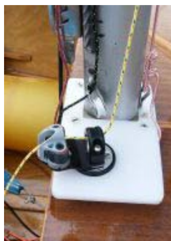
Figure 14: Steve Blackburn's original extended step. Steve now uses a similar commercial step which is 35mm wider than a conventional mast step.
